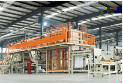
▲ BNBM Waterproofing's polymer membrane production line
